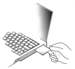
10. Slide the CardBus Adapter completely into the PCMCIA CardBus slot. Windows XP will detect new hardware and install the Wireless CardBus Adapter automatically. 11. Continue with "Using the IBM Client Utility to set up your wireless network under Windows XP, Windows 2000, and Windows NT 4.0" on page 9.
